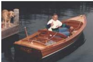
The base hull is built with western red cedar bead & cove planking, fiberglass and epoxy. The motor, batteries, solar panel kit, hardware and fittings can be ordered with the kit or separately. We will consult with you on your specific
