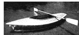
lbs. Easily paddled or rowed and perfect for quiet lakes and rivers. Using a taped seam method with three plywood frames makes this an easy to build and low cost project. Full-sized patterns, instructions and plans for paddles or oars. Plans (Item **Clkp**) Basic Kit (Item **Clk**).
