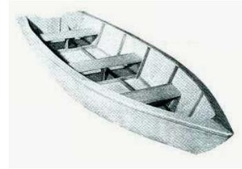
and rowed. Plywood used in the hull and the sheer covering boards not only complement but add significant strength. Utility Skiff 12' Plans (Item **Dctlhkp**); Basic Kit (Item **Ctlhk12**) Utility Skiff 14' Plans (Item **Dctlhkp**); Basic Kit (Item **Ctlhk14**).
