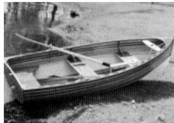
The hull design offers a traditional look with durable wood strip and epoxy. Easily car topped, towed or lifted on a deck. For handy references, see Ted Moores' *CanoeCraft or Rip, Strip and Row* by Harstock.
