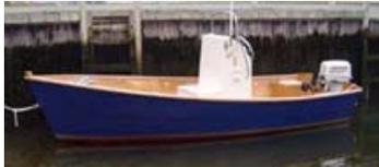
The bow design keeps this boat very dry, reduces pounding and allows it to bank on turns. It also makes building easy and fast. Construction is epoxy and plywood with stitch & glue, no jig or difficult framing is required. Plans for all hull parts and console. Rated up to 35 hp. Plans (Item **Coutp**) Basic Kit (Item **Cout**)
